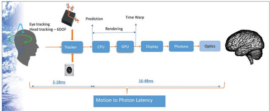
Figure 2: Six Degrees of Freedom (DOF) offers more than orientation (3 DOF), but will track your location as you physically move around. Latency (lag) adds up as the XR system collects and processes huge amounts of data. (Source: TDK InvenSense.)
